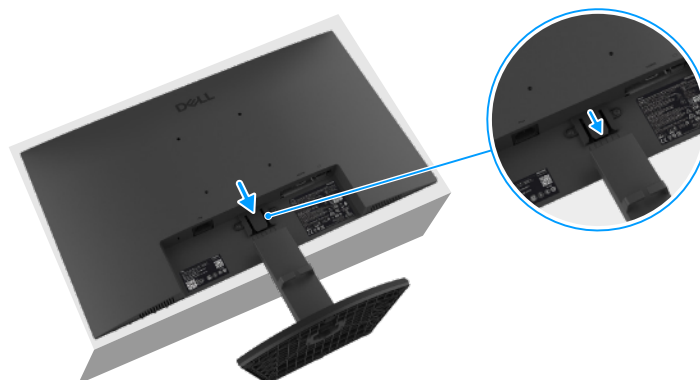
Figure 21. Remove the stand
